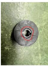
4. It could be minor adjusted as per your preferance after assembling on car. Clockwise: the shoes get tightened and transmit to 2nd speed slower Counter-clockwise: the shoes get loosen and transmit to 2nd speed faster
